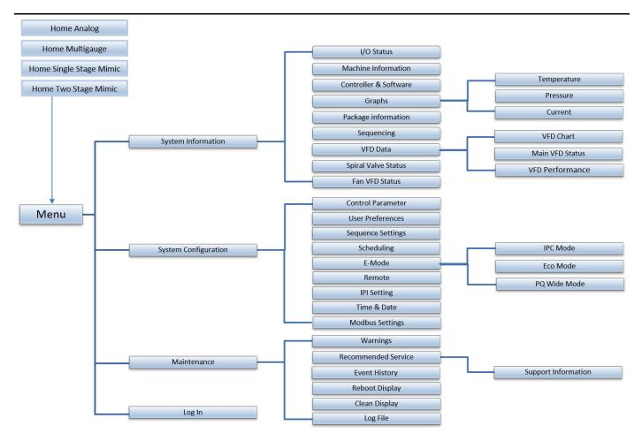
Figure 6-5: Sullair touch screen controller menu hierarchy
