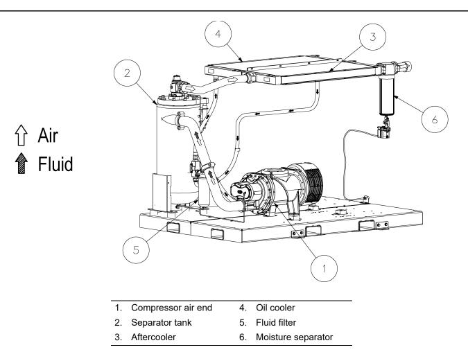
Figure 2-2: LS90 and LS110 cooling / lubrication and discharge system
